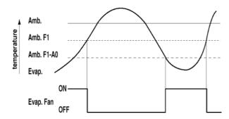
When 'F0'=2, parameter 'F1' indicates the absolute temperature for starting the fans.
