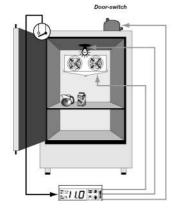
**Note:** If the light was previously switched on manually, when the door is closed the second time, it is automatically switched off.
