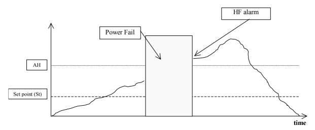
The activation of one or both of the alarms causes the  $^{\text{\tiny{MCP}}}$  LED to flash and the display of the alarm code, as well as the recording of the alarm to the E<sup>2</sup>PROM and the activation of the alarm relay or buzzer (if present).
